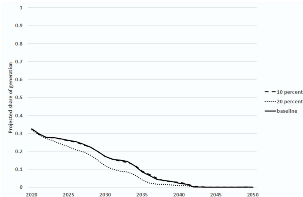
Figure 5 Projected global coal share of generation under the SDS-equivalent and Asian scenarios
