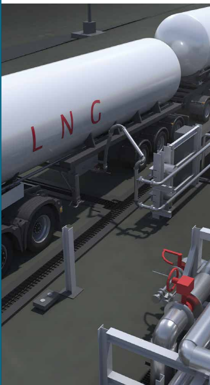
Schematic (not to scale) of the LNG truck-loading facility at Pluto LNG.
