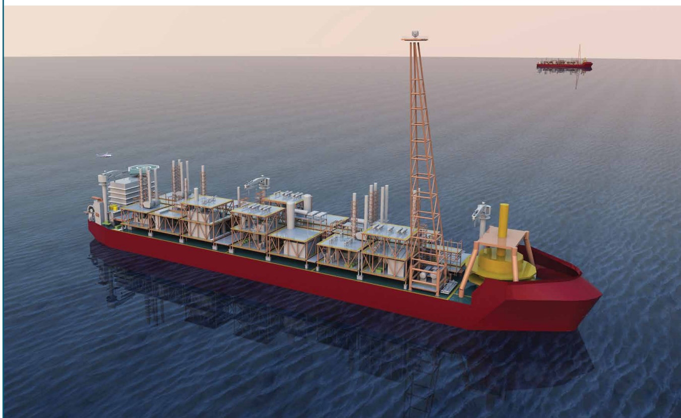
Indicative gFPSO facilities for the Browse development (schematic not to scale).
