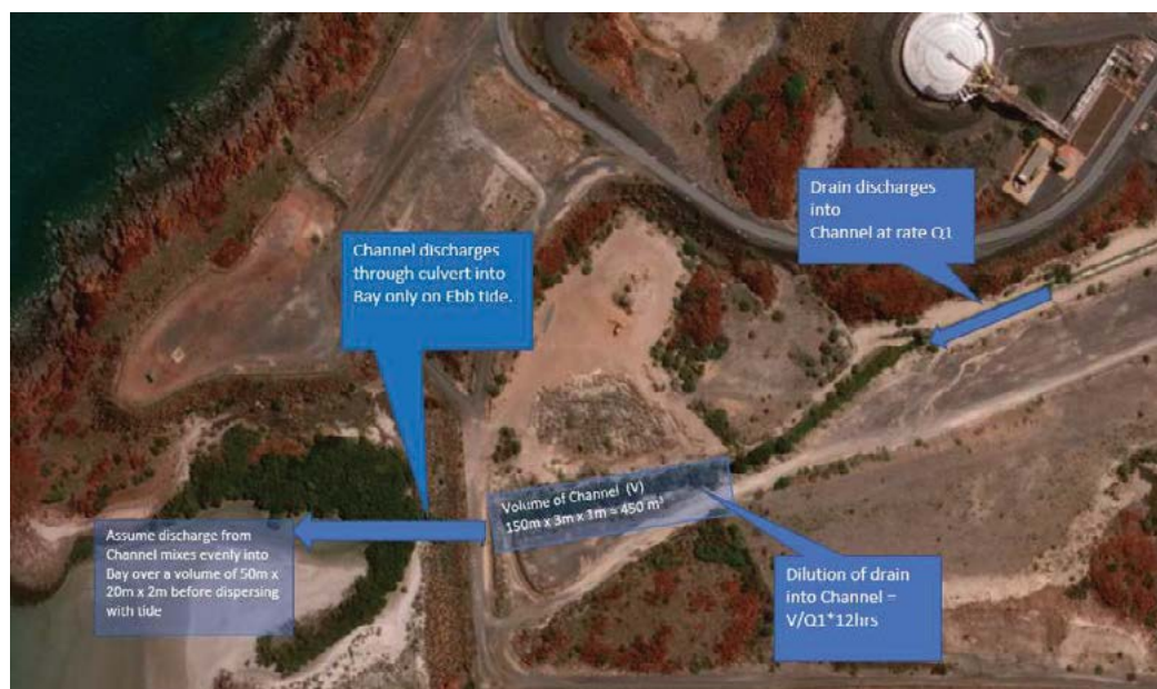
Figure 6-1: Schematic of Admin Drain discharge.
