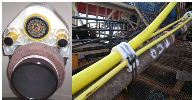
Figure 2. Minerva Pipeline Bundle Arrangement
