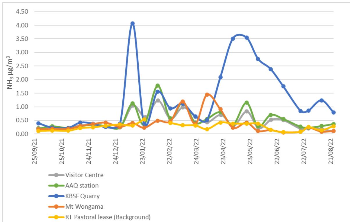
**Figure 3.5: Measured 15 day average  $\text{NH}_3$  by Radiello sampling**
