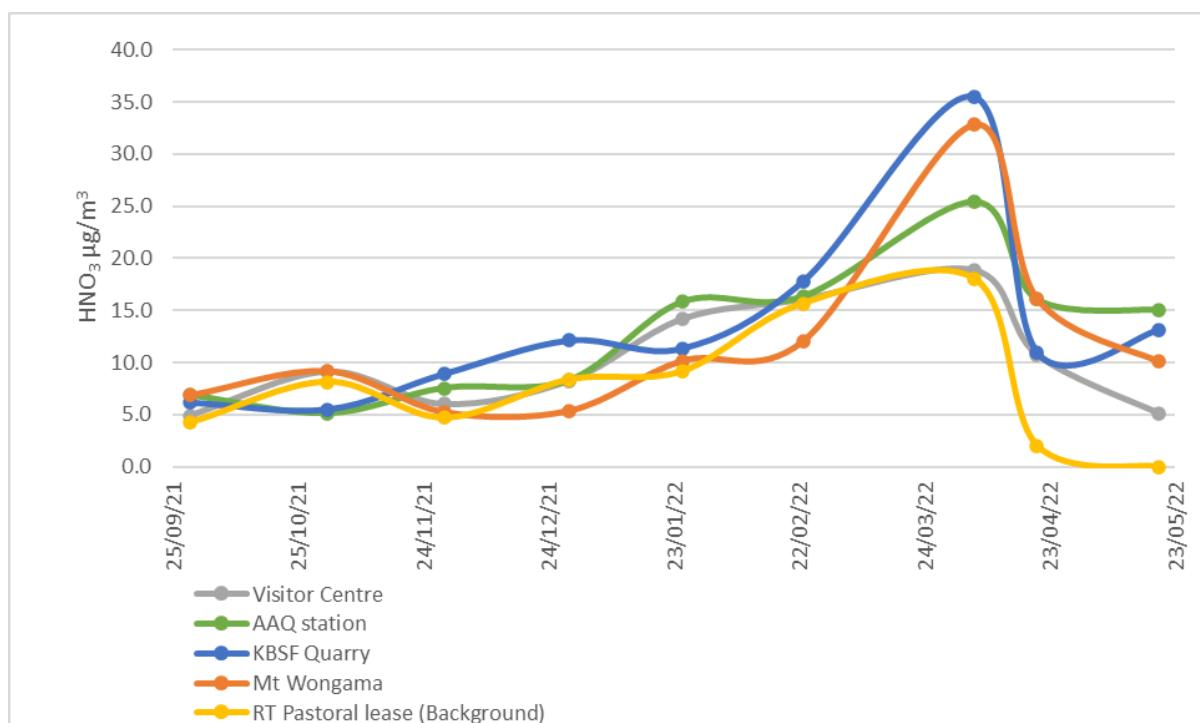
**Figure 3.7: Measured 30 day average  $\text{HNO}_3$  by Gradko sampling**
