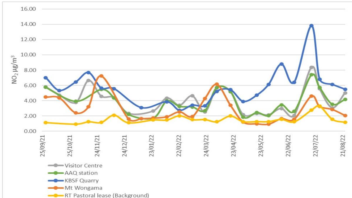
**Figure 3.1: Measured 15 day average  $\text{NO}_2$  by Radiello sampling**
