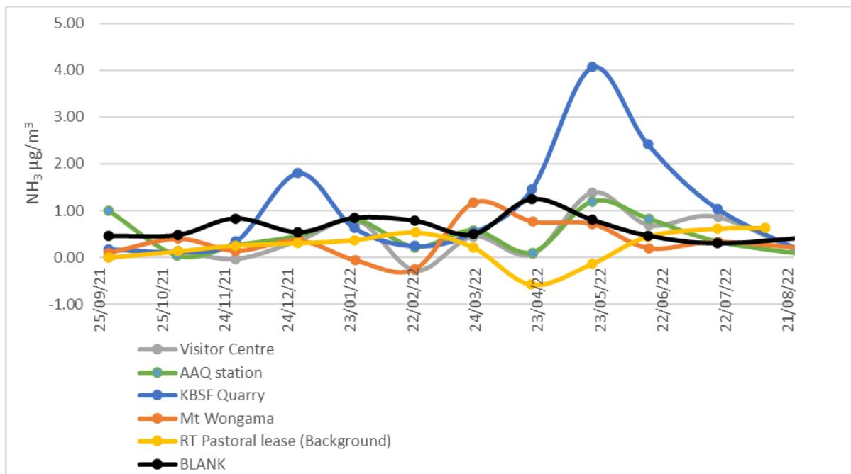
**Figure 3.13: Measured 30 day average  $\text{NH}_3$  by Ferm sampling**
