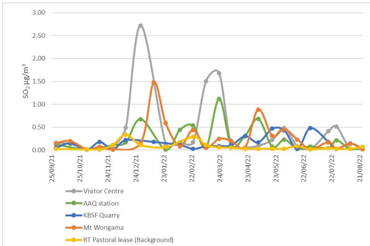
**Figure 3.4: Measured 15 day average  $\text{SO}_2$  by Radiello sampling**
