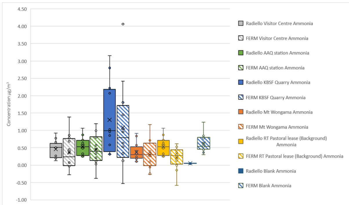
**Figure 3.18: Comparison of NH<sub>3</sub> Radiello and Ferm 30 day average datasets**
