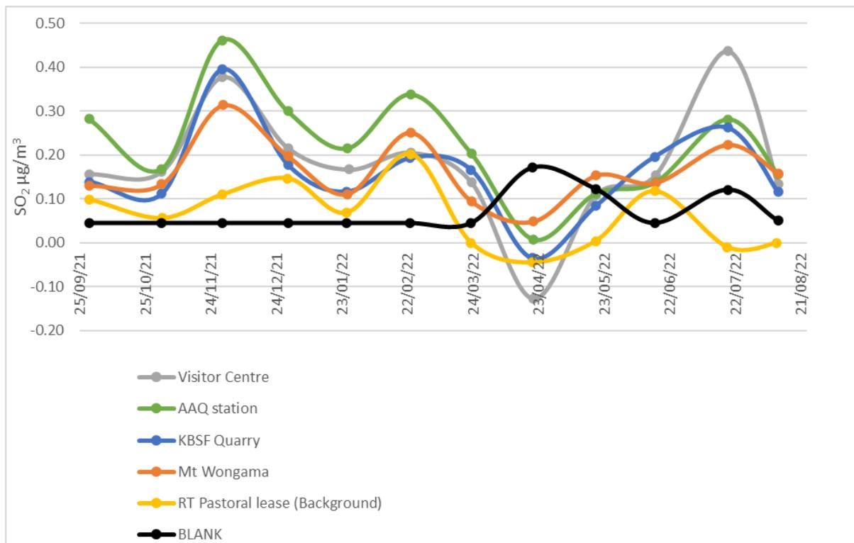
Figure 3.12: Measured 30 day average  $\text{SO}_2$  by Ferm sampling
