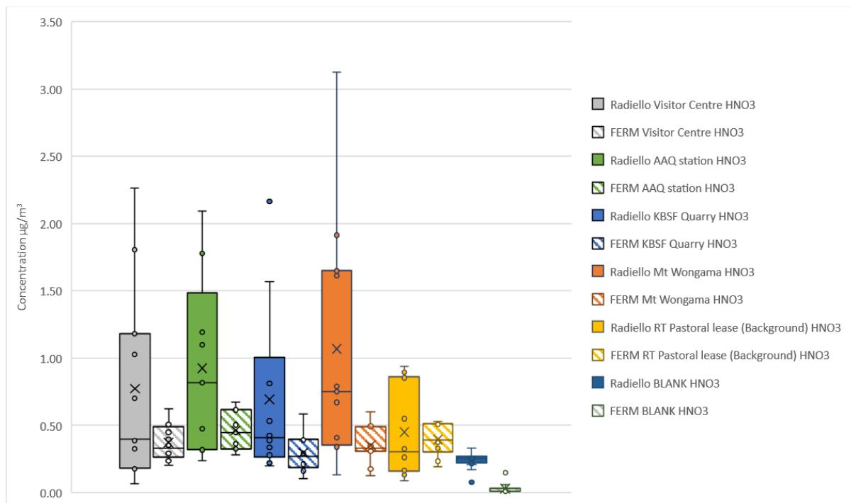
**Figure 3.17: Comparison of HNO<sub>3</sub> Radiello and Ferm 30 day average datasets**
