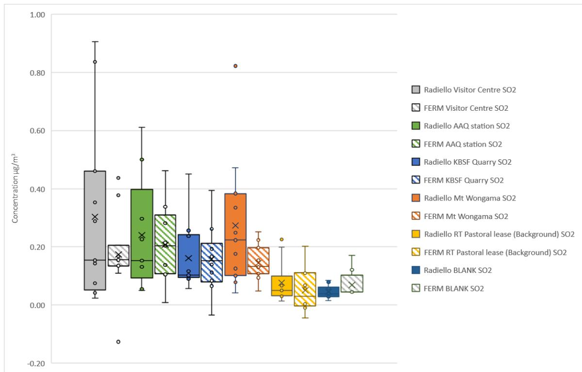
**Figure 3.16: Comparison of SO<sub>2</sub> Radiello and Ferm 30 day average datasets**
