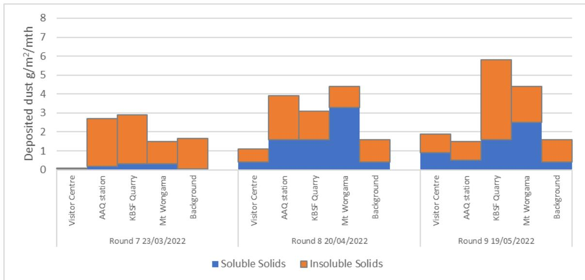
**Figure 3.40: Deposited dust 23 March 2022– 15 June 2022**
