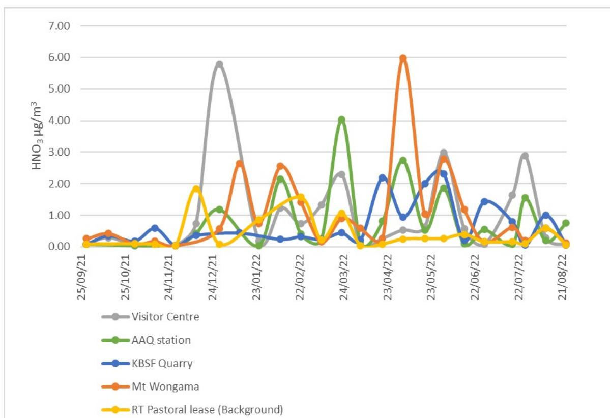
**Figure 3.3: Measured 15 day average HNO<sub>3</sub> by Radiello sampling**
