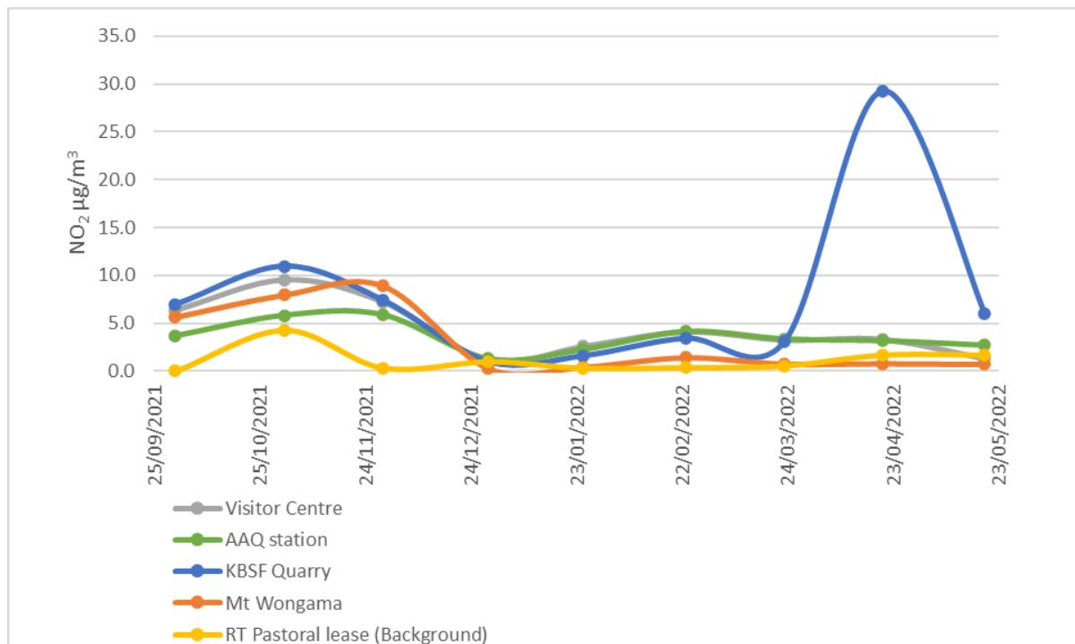
**Figure 3.6: Measured 30 day average  $\text{NO}_2$  by Gradko sampling**
