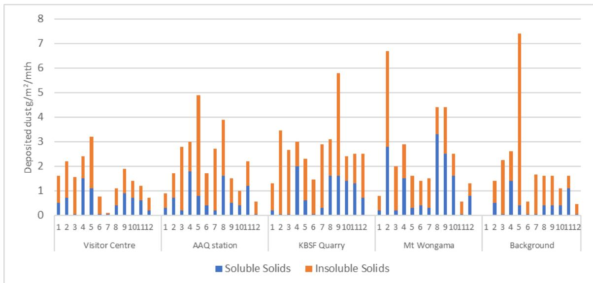
**Figure 3.42: Deposited dust data site trends across the twelve sampling rounds**
