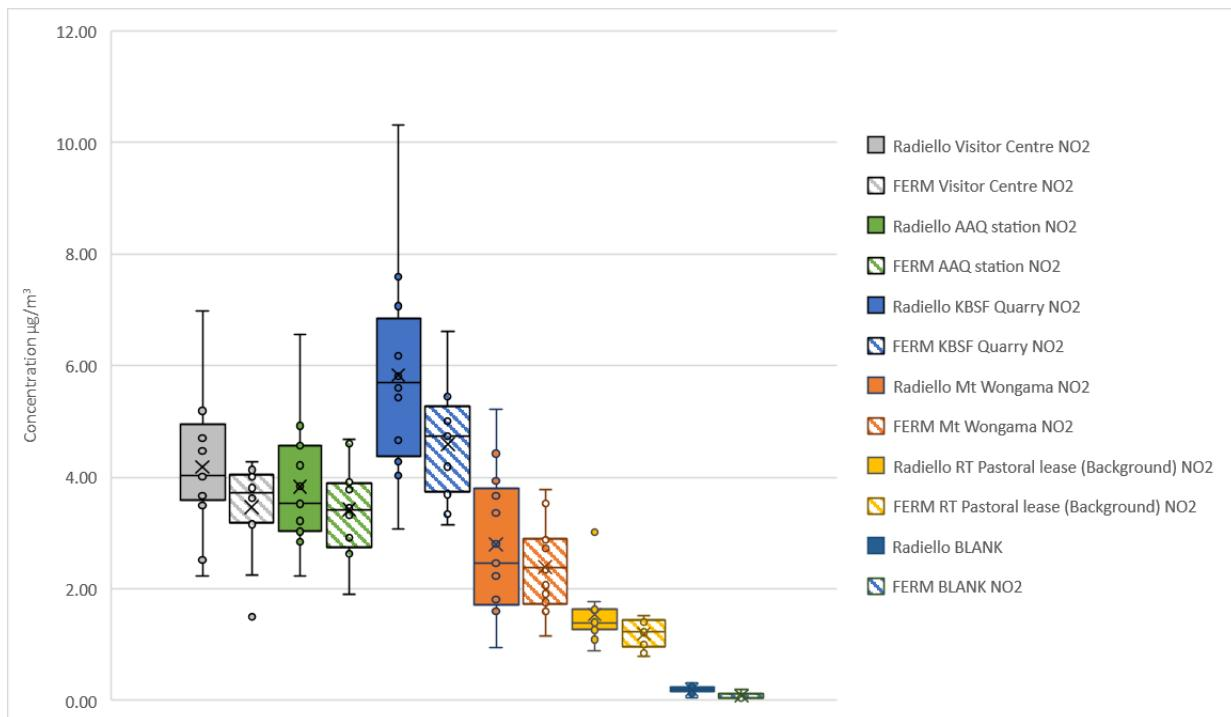
**Figure 3.14: Comparison of  $\text{NO}_2$  Radiello and Ferm 30 day average datasets**
